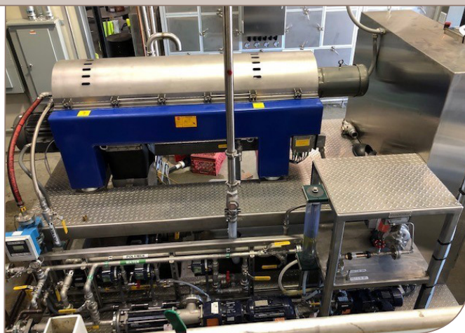
Hollandia chose an Alfa Laval ALDEC 20 decanter centrifuge to dewater its dairy wastewater biosolids prior to further processing. Alfa Laval was chosen not only for its proven technology, but for its partnership and expertise in wastewater treatment.
