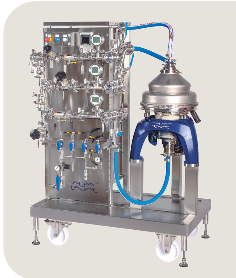
design. The machine can be configured for different separation duties, different disc angles and different solid/heavy phase removal by different conversion kits. The Alfa Laval Explorer can be configured for two-phase separation as well as three-phase separation, with solids removal by discharge or using the Alfa Laval TopStream technology for continuous solids/heavy phase removal.
