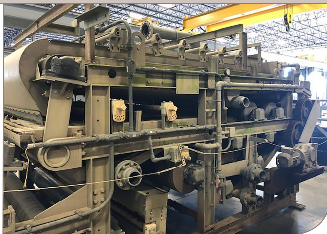
An example of an Alfa Laval AS-H belt filter press prior to rebuild (Alfa Laval service center photo)
