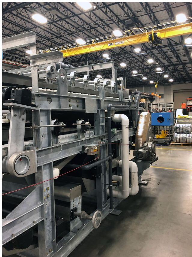
An example of an Alfa Laval AS-H belt filter press after refurbishment (Alfa Laval service center photo)
