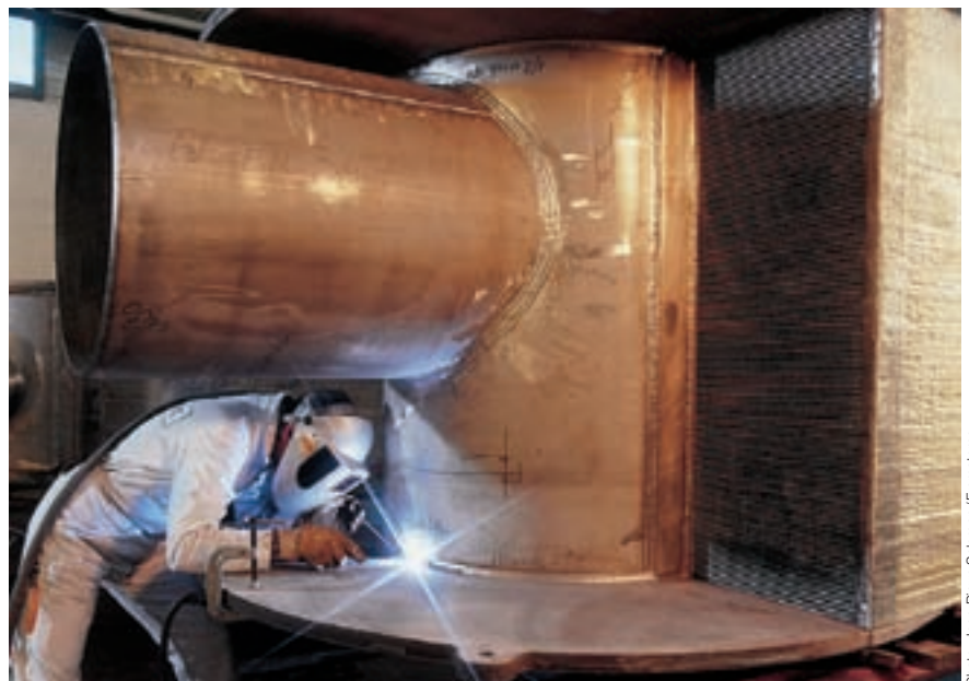
Welding of the effluent header to the plate bundle
