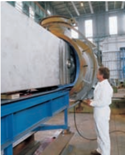
Insertion of the plate bundle into the pressure vessel is closely monitored
