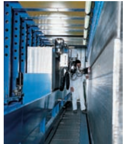
Inside the world's largest bundle press, an operator checks the welding of the bundle wall
