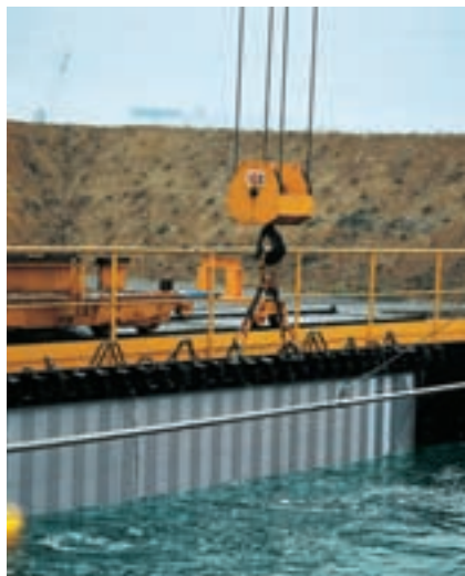
A newly corrugated plate emerging from the explosion forming pool
