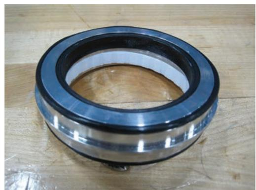
Mounting rotating nozzle and O-ring on upper plug:
