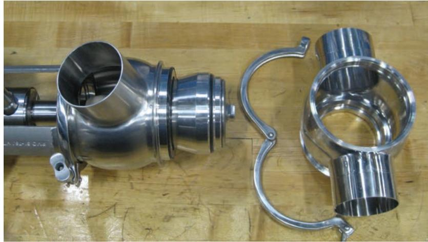
6. Remove flushing pipe using 19mm wrench.
