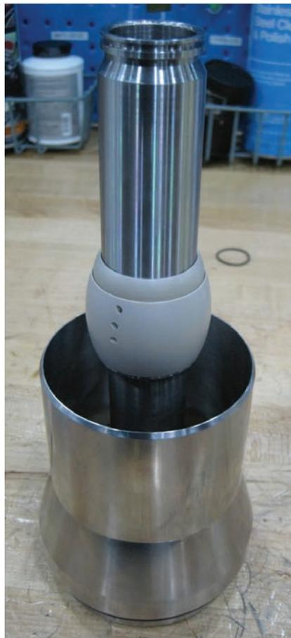
4. Nozzle and lock ring slides over spindle.
