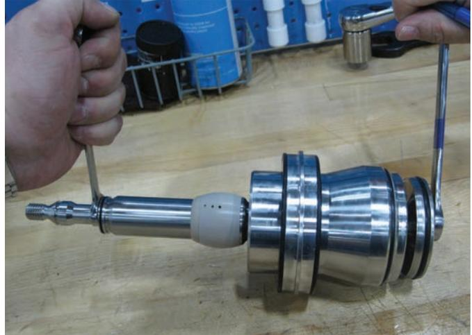
14. Tighten. Use a 13mm and 16mm wrench.
