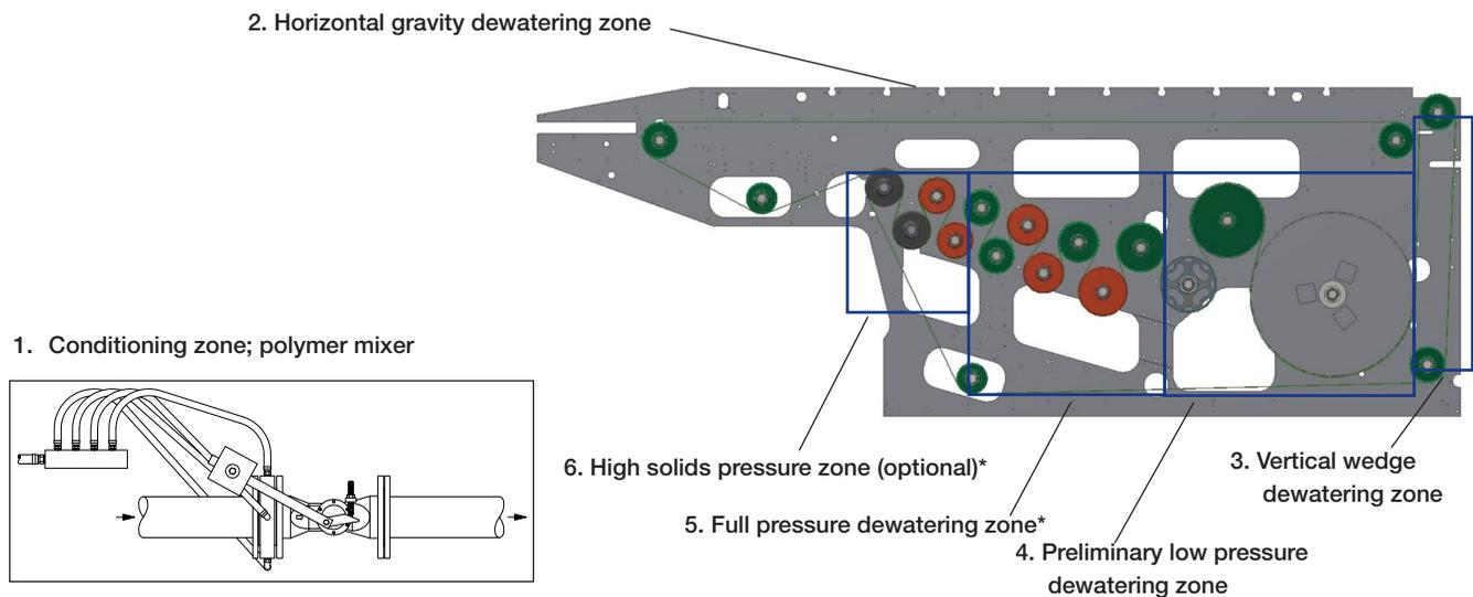
1. **Conditioning zone** – optimized dewatering begins with the proper conditioning of the slurry. Each unit is equipped with a proprietary variable orifice in-line polymer mixer that combines polymer and slurry instantly to facilitate rapid flocculation. This design allows the unit to use the lowest dosage of polymer while achieving the highest cake solids.
