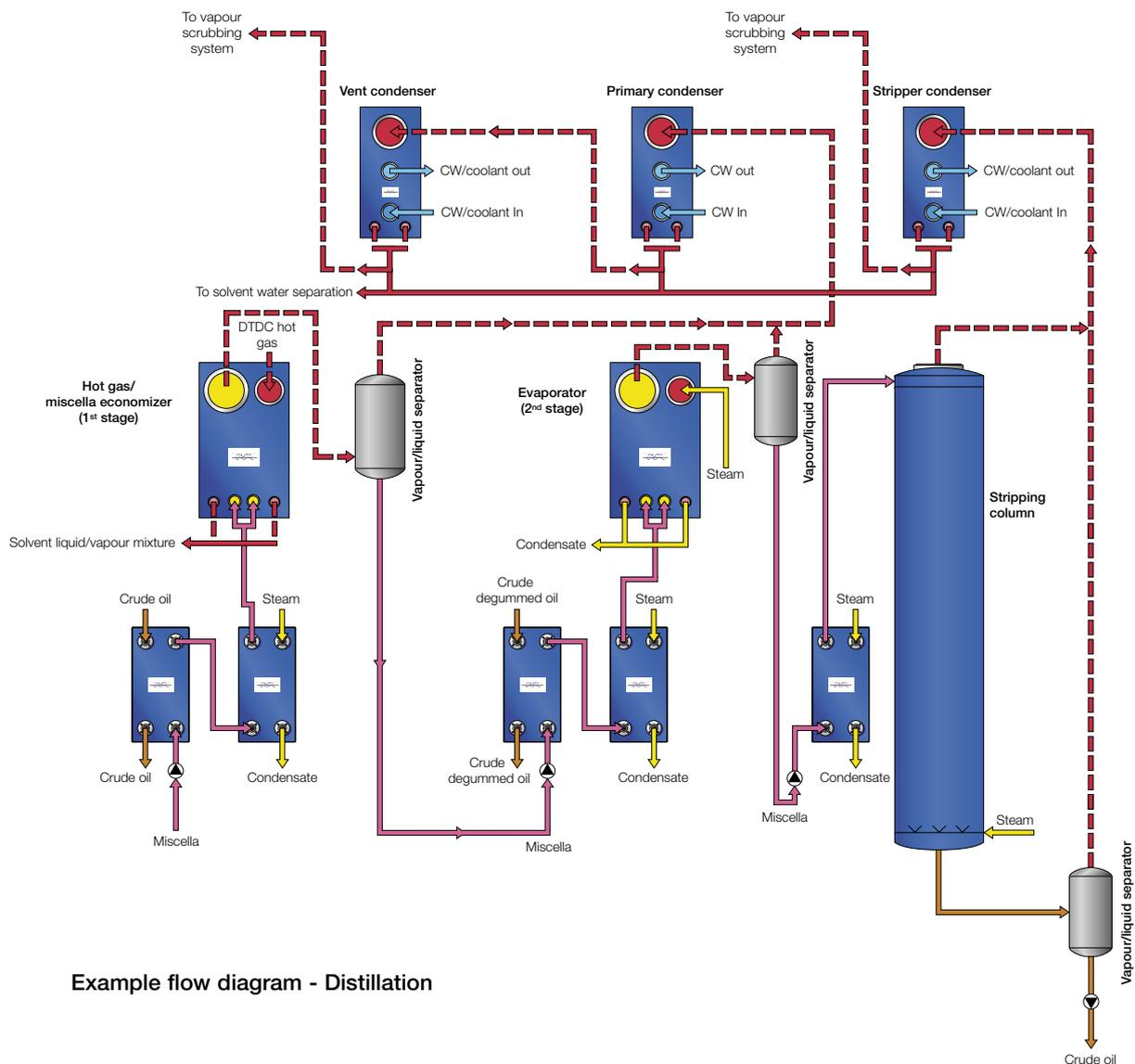
Example flow diagram - Distillation
