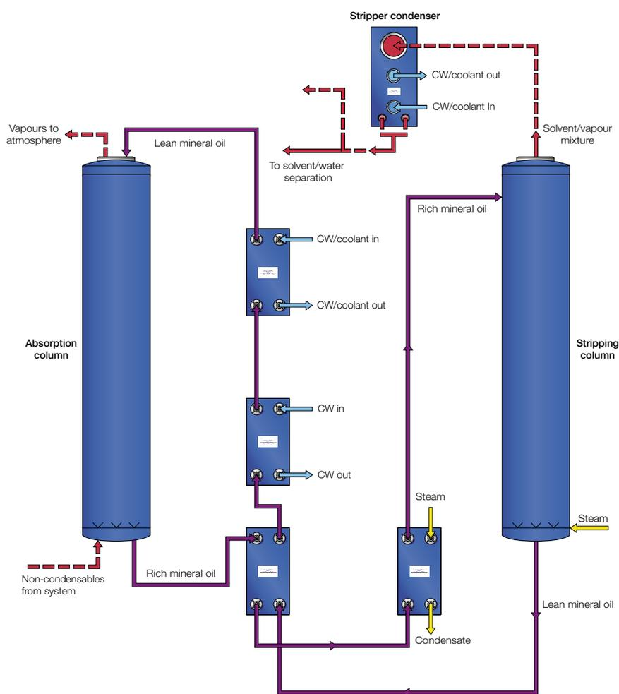
Example flow diagram – Vapour scrubbing
